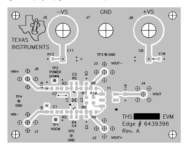
Figure 5–2. Bottom Layer 2 (Ground and Signal)
